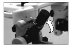
**5.1.3** Centric fixation (4.1) locked To lock the centric fixation completely, e.g. if the articulator has to be transported, or if no movements are desired, pull the joint axis into the precisely defined, final position.
