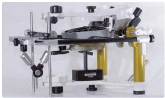
The maxillary model is oriented according to the mandible by means of the intraoral registration (functional impressions with secured Gnathometer M) and articulated accordingly.
