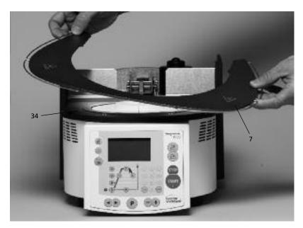
Secure the cooling tray (34) with the two screws (35) including the silicone washer (47).
