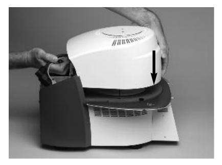
Ensure that the furnace head mounting mark (41) is aligned with the furnace base mounting mark (42).
