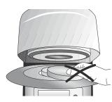
Never place objects in the firing chamber by hand, since there is a burn hazard. Always use the tongs (accessories) supplied for this purpose. Never touch the hot surface of the furnace head, as there is a burn hazard. Please also refer to the warnings on the furnace.
