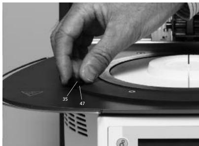
Step 2: Placing the firing plate (5)
