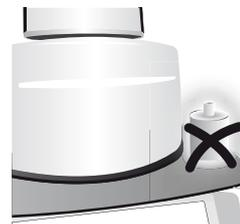
Do not cool the hot investment ring on the cooling tray. Use only the cooling grid for that purpose.
