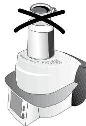
Foreign objects must not be placed on the furnace head or air vents. Make sure that no liquids or other foreign objects enter the air vents, since this may result in an electrical shock.
