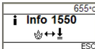
This information is only shown if the operation mode has been changed. Make sure that the furnace runs at the new stand-by temperature long enough before you start a program.
