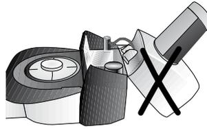
The furnace head should not be removed from the furnace base as long as the furnace head is connected by means of the heater cable.
