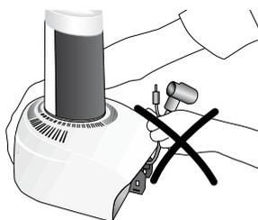
Do not carry the furnace head by the cables, since the cables and connections may be damaged.
