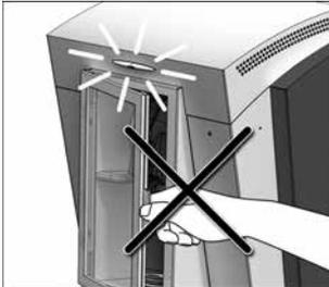
The safety door must not be opened while a program is in progress.
