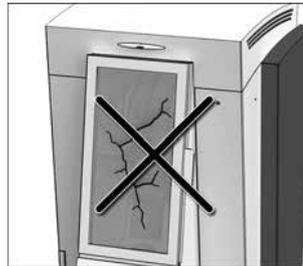
The injector must not be operated if it shows visible damage, for example, at the heater, safety door or clasps, etc.
