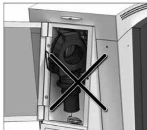
Make sure that the flask is correctly positioned. The injection program must not be started if the flask is incorrectly positioned.
