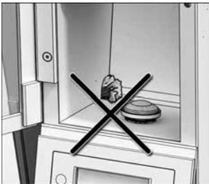
If the discharge outlet is clogged, the injector must not be operated.
