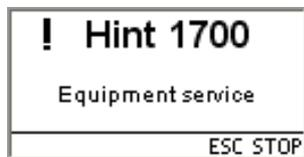
During operation, the injector continuously monitors all the functions. If an error is detected, the respective error message is displayed.
