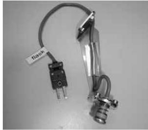
**Mounting the temperature sensor:**
