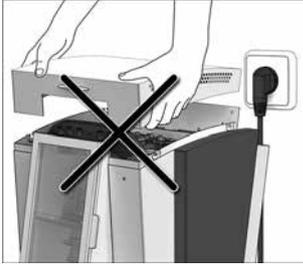
The hood may only be removed while the injector is switched off and the power plug disconnected.
