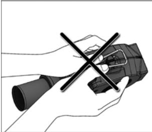
The locking clasp may only be removed from the flask by rotating, rather than pushing it.
