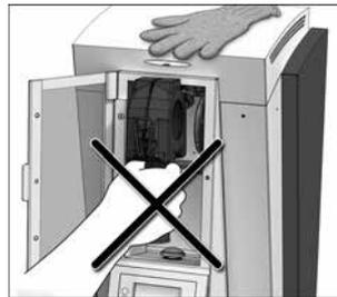
The flask must not be loaded or removed from the injector without thermal glove.
