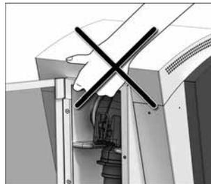
The injector may only be carried by supporting the bottom under the operating field and by the recessed grip at the rear of the injector.
