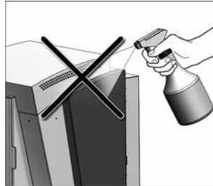
Make sure that no liquids or other foreign substances enter the injector during cleaning.
