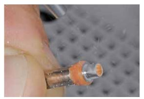
Carefully blast the bonding area with  $Al_2O_3$  (50–100  $\mu m)$  at low pressure until an even, smooth surface has been achieved.
