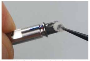
Clean in an ultrasonic bath or with a steam cleaner and then dry with blown air.
