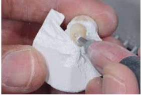
Fine divestment of the abutment crown is carried out with polishing beads at 2 bar (29 psi) pressure.
