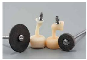
Separate the sprues using a separating disc. Avoid overheating.
