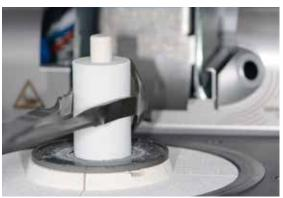
Then, place the side of the IPS Alox Plunger which has been coated with Separator into the  ${\rm hot}$  investment ring.
