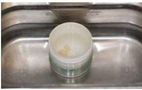
To remove the reaction layer, immerse the pressed objects in IPS e.max Press Invex ... and pla
