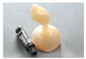
Possible rough spots interfering with the fit on the titanium bonding base cause stains on the screw channel of the pressed object ...
