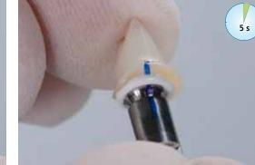
Subsequently, tightly press the components together for 5 seconds.
