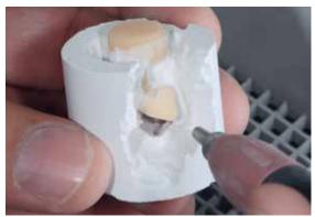
Rough divesting with polishing beads at 4 bar (58 psi) pressure until the object becomes visible.
