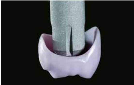
Select the largest possible IPS e.max CAD Crystallization Pin.
