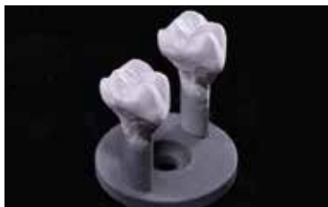
Secure the restoration on a suitable IPS e.max CAD Crystallization Pin as described in Variant B and C and apply IPS e.max CAD Crystall./Glaze Spray.
