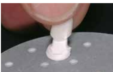
Remove the restoration from the set firing paste.
