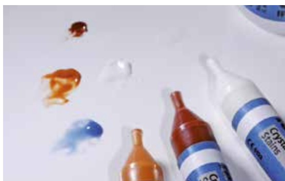
Extrude IPS e.max CAD Crystall./Shades and Stains from the syringe and mix thoroughly. If required, thin with IPS e.max CAD Crystall./Glaze Liquid.
