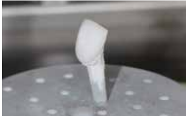
Place the restoration in the centre of the IPS e.max CAD Crystallization Tray and fire using the stipulated firing parameters.
