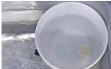
Remove residue with ultrasound in a water bath ...
