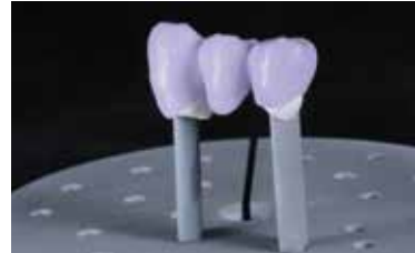
Place the restoration in the centre of the IPS e.max CAD Crystallization Tray and fire using the stipulated firing parameters.
