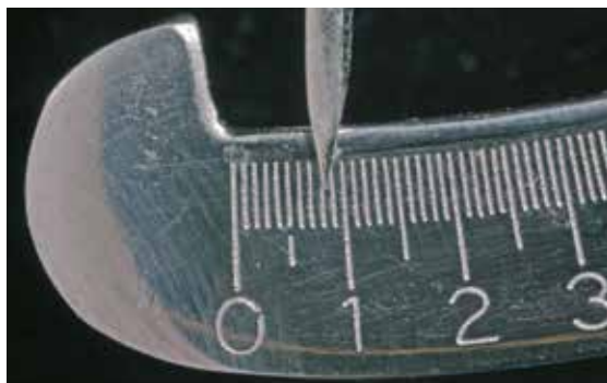
Make sure that the minimum layer thicknesses are maintained even after the minor adjustments.
