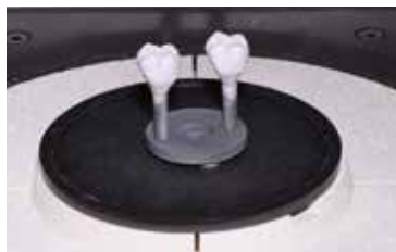
Position the IPS e.max CAD Speed Crystallization Tray with max. two IPS e.max CAD HT/MT/LT in the furnace and fire using the parameters for the Speed Crystallization firing.
