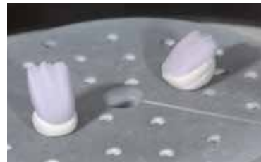
Place the firing tray in the furnace and start the Crystallization with the respective parameters.
