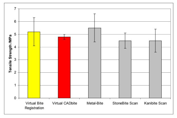
Fig. 5: Tensile strength values of different bite registration materials (R&D, Ivoclar Vivadent, 2007)
