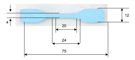
Fig. 4: Test specimen for tensile strength measurement
