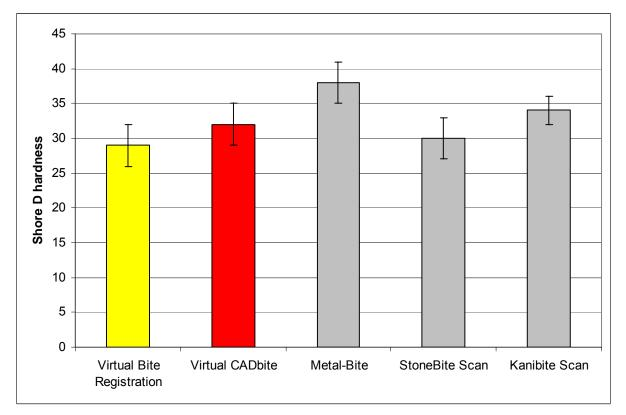
Fig.3: Shore D hardness of various bite registration materials (R&D, Ivoclar Vivadent, 2007)
