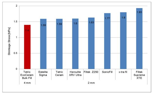
Furthermore, tests showed that the shrinkage force exhibited by a 4 mm increment of Tetric EvoCeram Bulk Fill was lower than that of 2 mm increments of other products.
