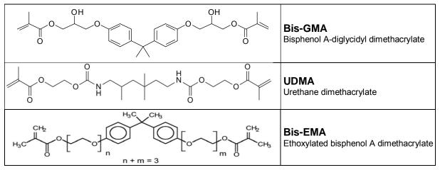
Table 2: Table illustrating the structural formulae for the monomers used in Tetric EvoCeram Bulk Fill
