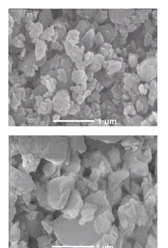
Fig. 1a,b: Barium aluminium silicate glass fillers with a mean particle size of 0.4  $\mu$ m (top picture) and 0.7  $\mu$ m (bottom picture) as used in Tetric EvoCeram Bulk Fill.
