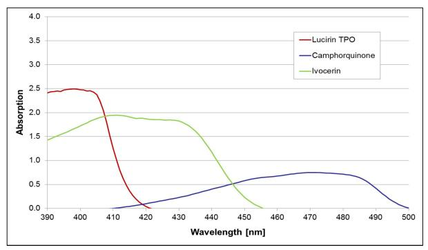
Fig. 11: Absorption spectra of Lucirin TPO, camphorquinone and Ivocerin<sup>®</sup> as measured in the laboratory. *(R&D Ivoclar Vivadent 2012)*
