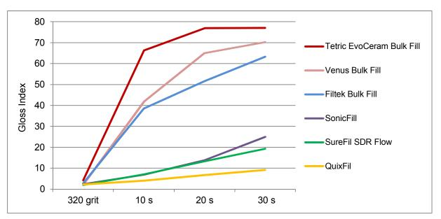
Fig. 31: Mean surface gloss of various bulk fill composite materials compared to Tetric EvoCeram Bulk Fill after polishing with OptraPol Next Generation in relation to polishing time. (*Preclinic R&D Ivoclar Vivadent, Schaan, August, 2011*)
