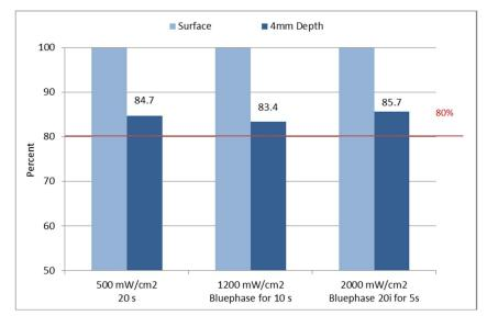
Fig. 17c: Tetric EvoCeram Bulk Fill **Shade IVW**: 4 mm depth hardness as percentage of surface hardness, measured with different light intensities
