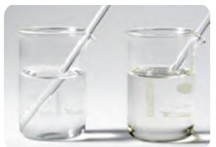
Fig. 5: Illustration of refractive index with glass rods in water (left) and monomer mixture with coordinated refractive index (right)
