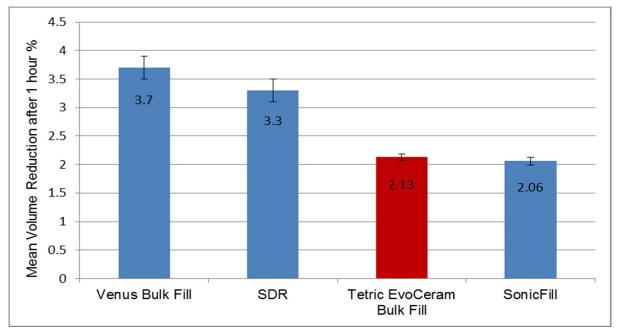
Fig. 24: Mean percentage of volumetric shrinkage after 60 minutes of different composites. (Dr C. Koplin, Fraunhofer Institut für Werkstoffmechanik IWM, Freiburg, Germany, 2011)
