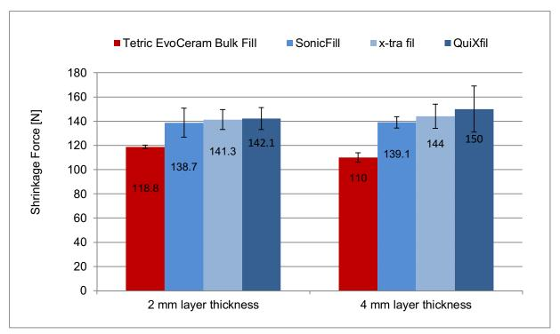
Fig. 25: Shrinkage stresses of various sculptable bulk fill materials measured in 2 mm and 4 mm layer thicknesses. *(K. Vogel, Abstract 858, AADR Poster, Florida 2012)*<sup>22</sup>
