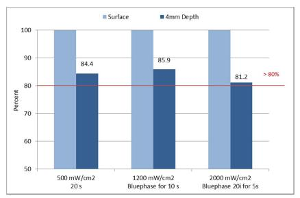
Fig. 17b: Tetric EvoCeram Bulk Fill **Shade IVB**: 4 mm depth hardness as percentage of surface hardness, measured with different light intensities
