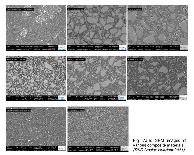
Apart from Filtek Bulk Fill/3M Espe (bottom, left) and Venus Bulk Fill/Heraeus Kulzer (bottom middle), all the other materials contain relatively large fillers. This correlates with the polishing results shown in section 4.5.
