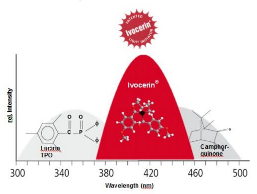
Fig. 10: Schematic representation of the absorption spectra of Lucirin TPO, Camphorquinone and  $\mathsf{Ivocerin}^{\texttt{®}}$
