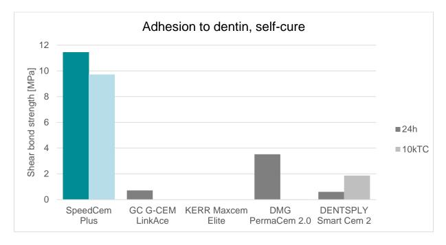
The shear bond strength was determined at a feed rate of 1mm/min.
