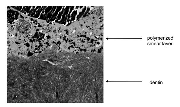
Fig. 3: TEM image of the interface between SpeedCEM and dentin (van Meerbeek, Leuven, 2009)
