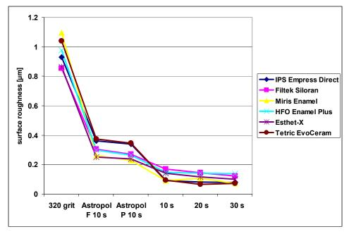
Fig. 12: Average surface roughness  $R_a$  (µm) of IPS Empress Direct and other composite restoratives after polishing with the three components of the Astropol polishing set (Astropol F, Astropol P and Astropol HP for 10, 20 and 30 seconds).
