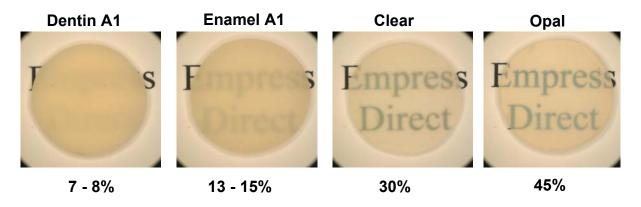
Fig. 7: Translucency of various IPS Empress Direct pastes illuminated from the front. The percentage indicates the amount of light that is transmitted through the materials.
