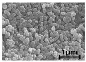
Spherical mixed oxide 150 nm
