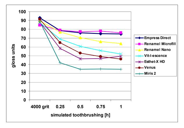
Fig. 14: Decrease in surface lustre of plane IPS Empress Direct specimens in comparison with conventional products after one-hour polishing with 4000-grit abrasive paper and 0.05-µm polishing medium, using Colgate Total toothpaste and contact pressure of 250 g
