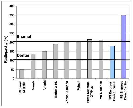
Fig. 10: Radiopacity of IPS Empress Direct Enamel and Dentin materials (blue) compared with that of conventional materials. The bold horizontal lines indicate the radiopacity of natural dentin (100% AI) and natural dental enamel (200% AI).
