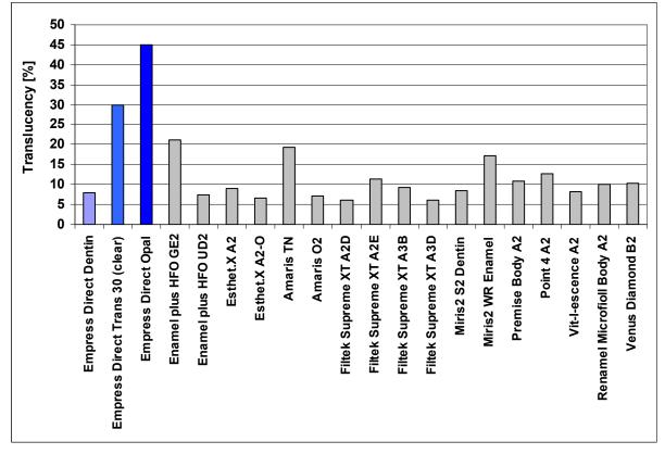
Fig. 8: Translucency of the different IPS Empress Direct materials compared to that of conventional products
