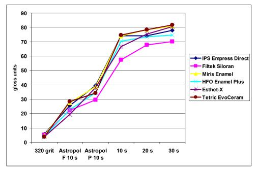
Fig. 11: A comparison of the average gloss of IPS Empress Direct and other composite restoratives after polishing with the three components of the Astropol polishing set (Astropol F, Astropol P and Astropol HP for 10, 20 and 30 seconds). Reference material: black glass = 94.2 gloss units
