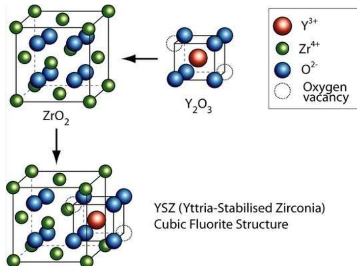
Figure 5: Stabilization mechanism and formation of oxygen vacancies by doping  $ZrO_2$  with  $Y_2O_3$  <sup>2</sup>.
