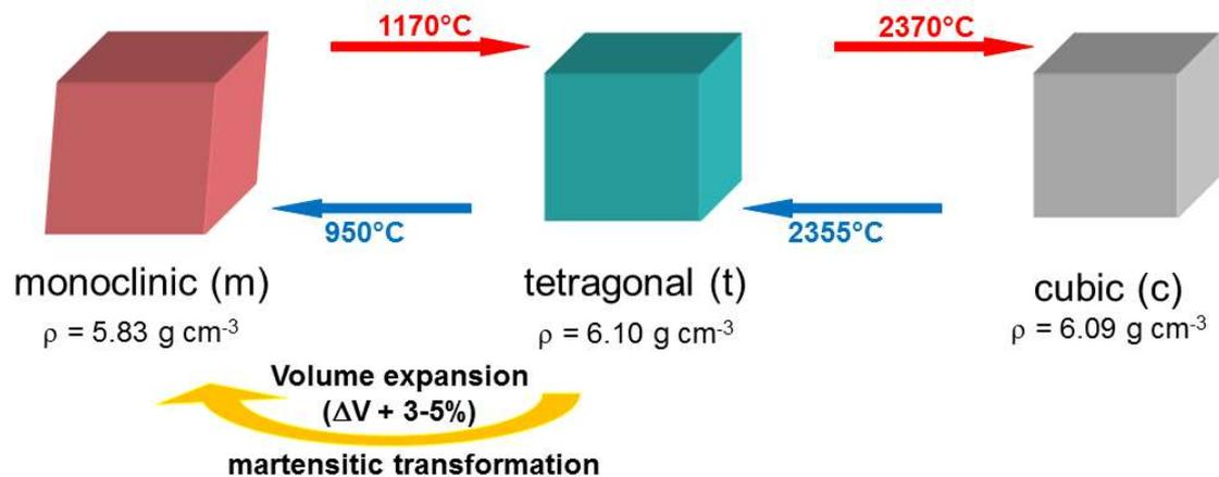
Figure 4: Correlation between temperature and volume change due to lattice transformation of the phases of zirconia.
