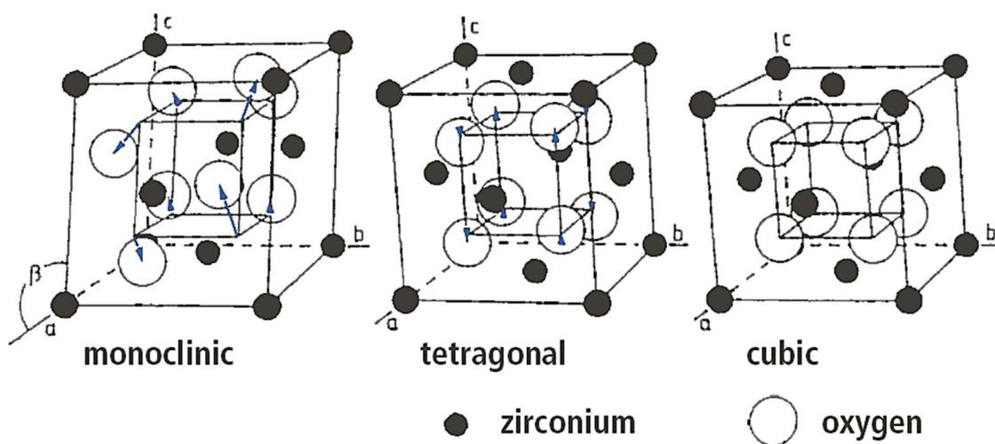
Figure 3: Three crystal structures of zirconia: monoclinic, tetragonal and cubic. The transformation from the cubic to tetragonal phase is associated with a stretching of the position of the oxygen ions along the c-axis. The tetragonal phase transforms into the monoclinic phase by an additional shearing of those ions (see direction of arrows) (adapted from [5]).
