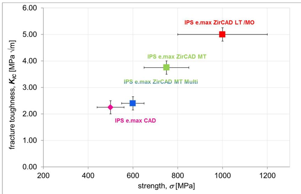
Figure 13: Comparison between different zirconia types (blue, green and red squares) and IPS e.max CAD (pink square). The influence of increasing yttria content on fracture toughness and strength is evident.
