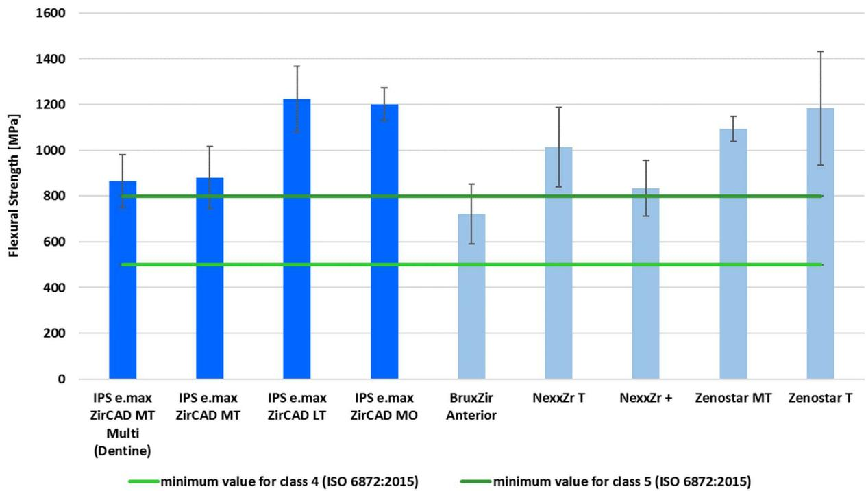
Figure 14: Comparison of flexural strength values of various IPS e.max ZirCAD products and competitor materials. The minimum values according to ISO 6872:2015 are shown as green lines.
