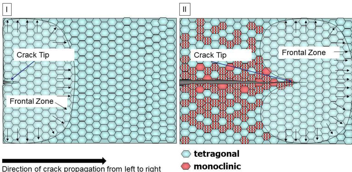
Figure 6: Scheme of transformation toughening in Y-TZP due to initial crack formation.
