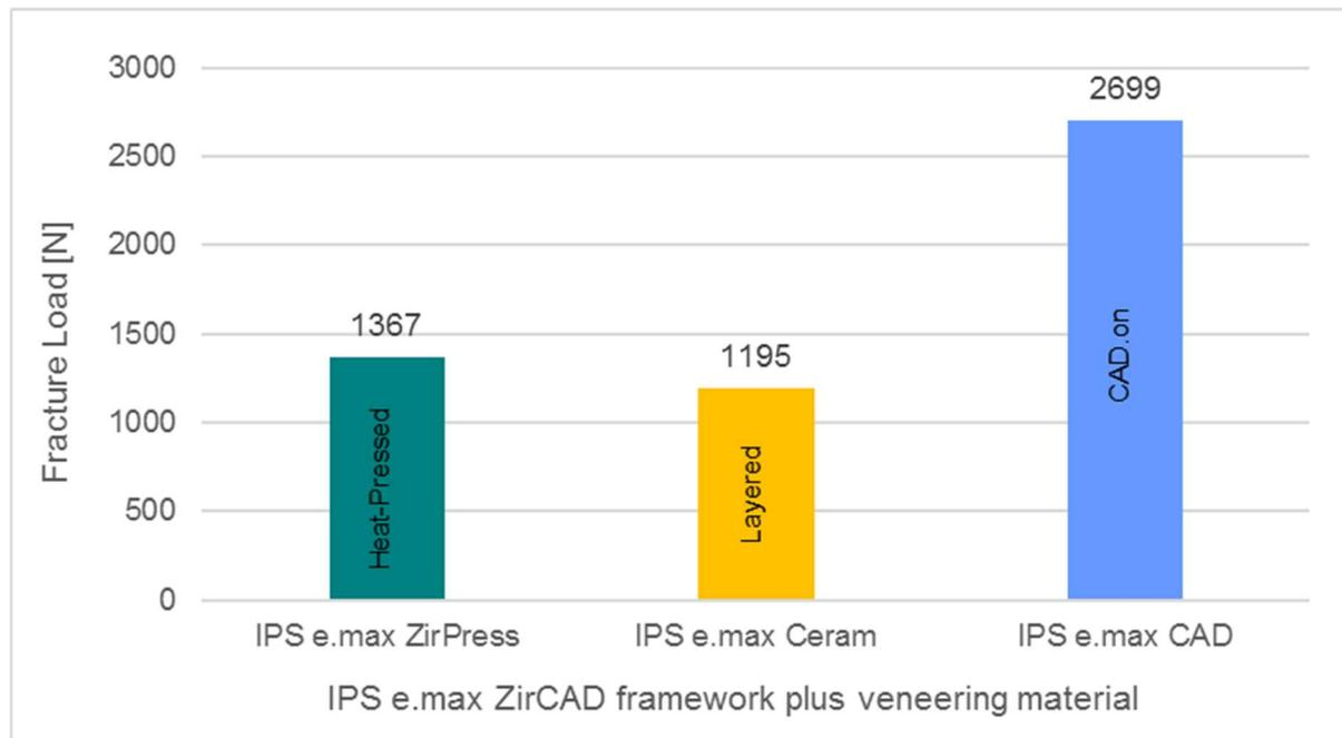
Figure 18: Single load to failure results of IPS e.max ZirCAD framework with different ceramic veneering structures applied using the press-on, layering and IPS e.max CAD-on techniques.
