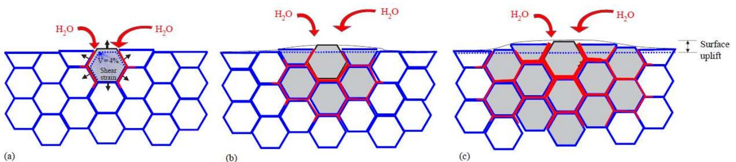
Figure 7: Schematic representation of the aging process. Starting from a single grain at the surface (a) followed by a cascade of transformations neighbour-to-neighbour (grey zone), leading to micro-cracking (water penetration along the red track) and surface roughening (b and c) (adapted from [12]).
