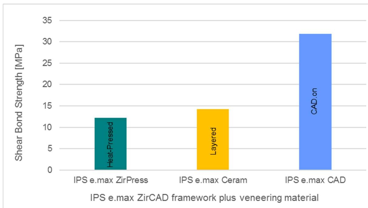
Figure 19: Shear bond strength of IPS ZirCAD frameworks with varying veneering structures.
