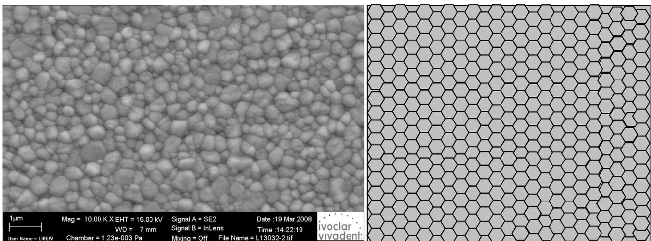
Figure 11: Micrograph of 3Y-TZP material and schematic illustration of uniform grains.
