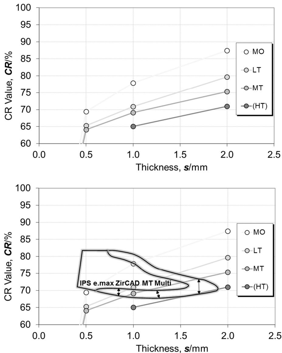
Figure 17: Dependence between opacity CR and wall thickness. In the lower graph, the cross section of an anterior IPS e.max ZirCAD MT Multi crown indicates the concept of the translucency gradient. MO = medium opacity, LT = low translucency, MT = medium translucency and HT = high translucency.
