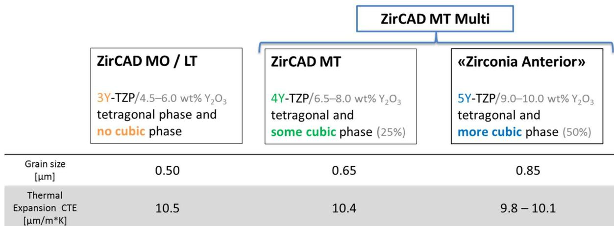
Figure 10: Overview of used types and characteristics of TZP materials within the IPS e.max ZirCAD portfolio.
