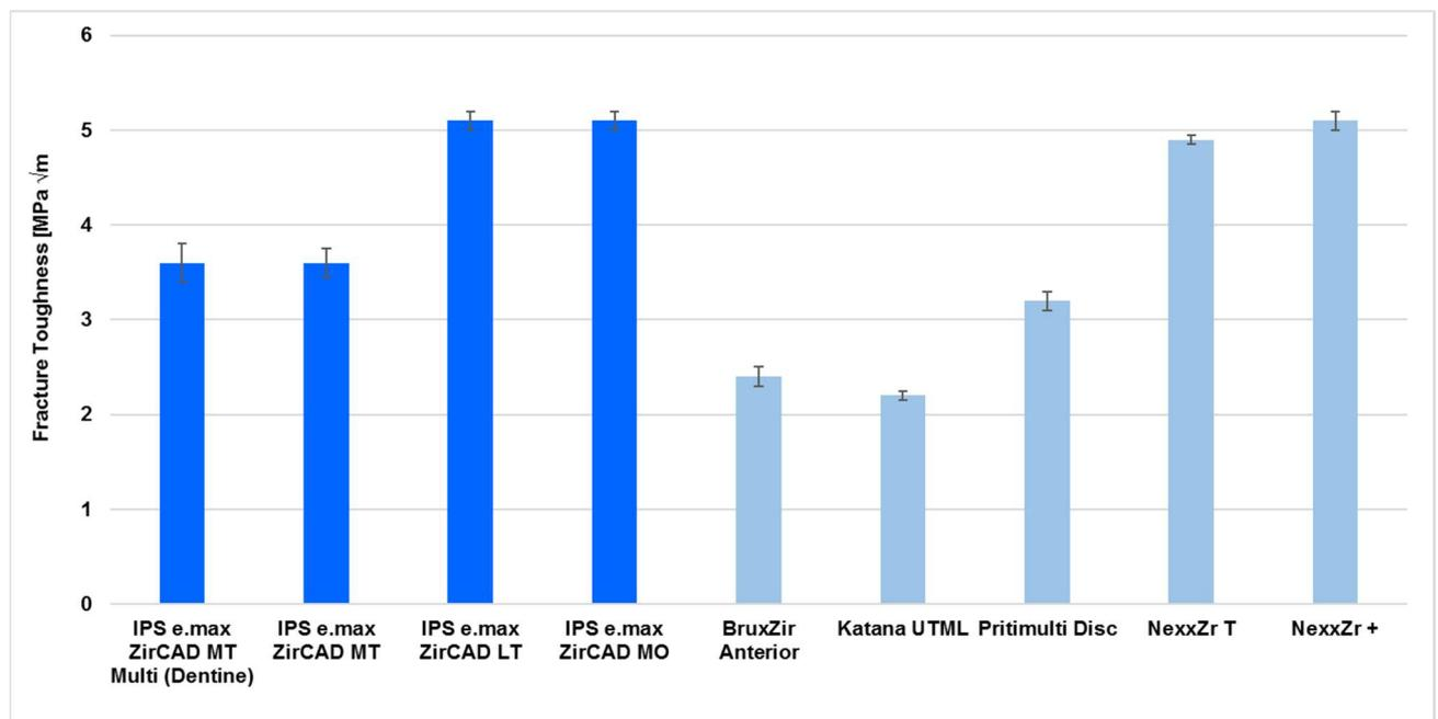
Figure 15: Comparison of fracture toughness values of various IPS e.max ZirCAD products and competitor materials.
