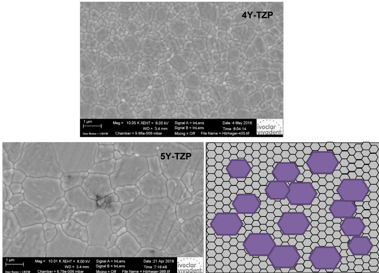
Figure 12: Micrograph of 4-Y-TZP (upper graph) and 5Y-TZP material and schematic illustration (lower graphs). The schematic illustration shows the 50:50 composition of tetragonal (grey) and cubic (purple) phase in 5Y-TZP.
