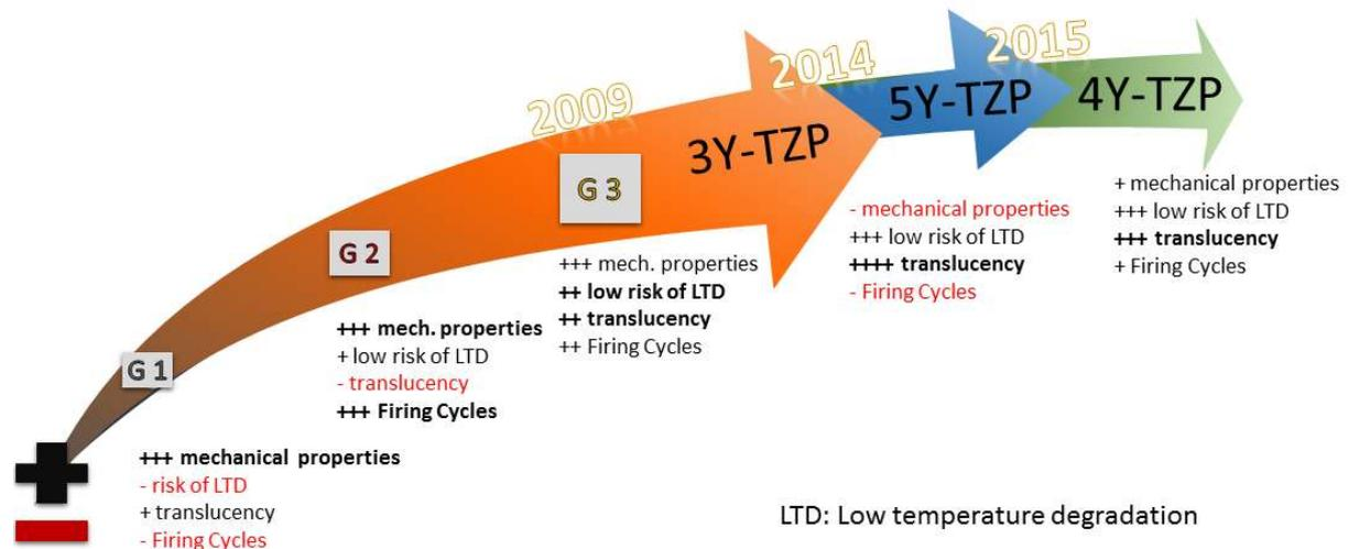
Figure 8: Evolution and characteristics of dental zirconia types: different generations of 3Y-TZP until 2014. After 2014 the 5Y-TZP materials were introduced to the dental market. Low temperature degradation (LTD) describes the aging sensitivity of zirconia.
