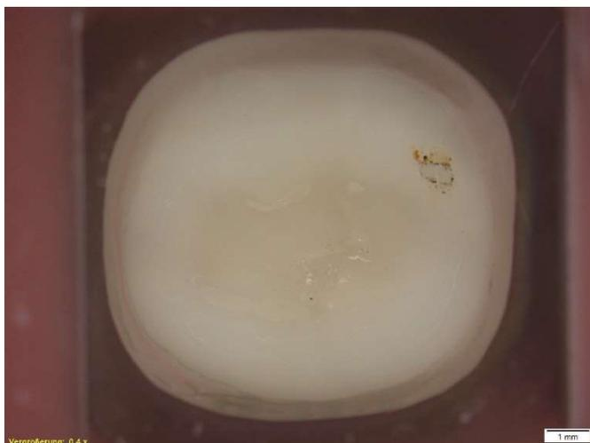
Figure 20: IPS e.max ZirCAD MT molar crowns after 200,000 dynamic loading cycles at 170N.
