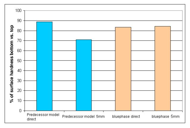
Fig. 13: Differences in the curing quality achieved with curing lights using different light guides (parallel vs. Turbo) at distances of 0 and 5 mm (Price, Halifax, 2007).
