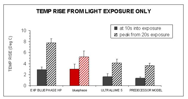
Fig. 29: Temperature increase after direct irradiation of the bottom of the cavity without composite (Rueggeberg, Augusta, 2007)
