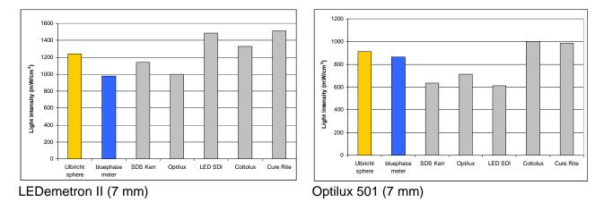
Fig. 32: Diagrams of the light intensities of four different curing lights measured by means of different radiometers compared to the integrating sphere.
