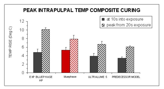
Fig. 28: Temperature rise after curing of the first composite increment using the High Power mode. (Rueggeberg, Augusta, 2007)
