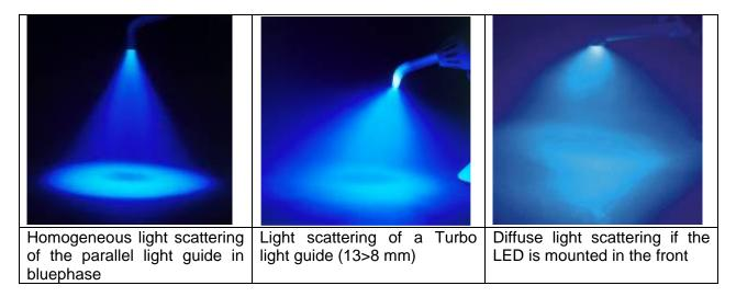
Fig. 7: Light scattering characteristics of different light guides
