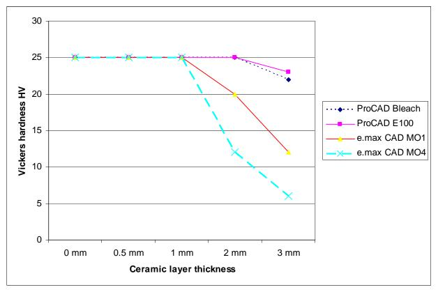
Fig. 23: Vickers hardness of Variolink II Base after curing through ceramic layers of various thicknesses (ProCAD and IPS e.max CAD) (Ilie, Munich, 2007)
