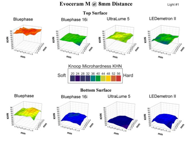
Fig. 16: "Surface Mapping" of the Knoop micro-hardness of Tetric EvoCeram after having been exposed to the light of different curing lights for 10 s. Distance of the light guide: 8 mm (Price, Halifax, 2007)
