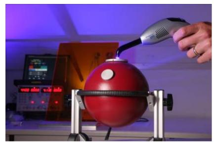
Fig. 9: Measurement with the integrating sphere
