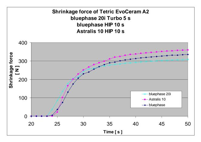
Fig. 22: Measurement of the shrinkage force of Tetric EvoCeram when cured with bluephase, bluephase 20i and Astralis 10 (Burtscher, Ivoclar Vivadent AG 2008).
