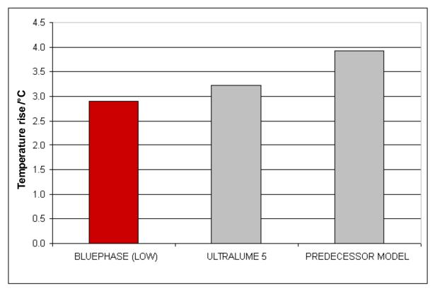
Fig. 27: Temperature increase after a curing time of 10 s in the curing mode for adhesives (Rueggeberg, Augusta, 2007)
