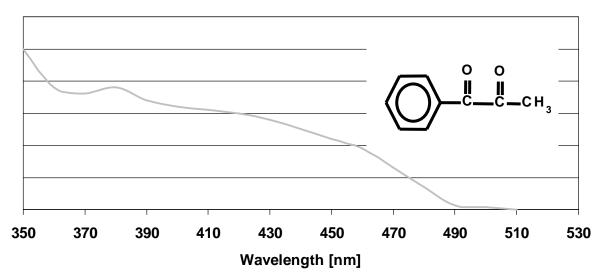
Fig. 2: Absorption spectrum of phenylpropanedione (PPD)
