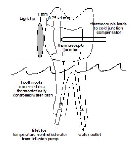
Fig. 24: Diagram of the temperature measurement in the pulp chamber when a buccal cylindrical cavity is irradiated.
