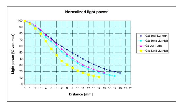
Fig. 6: Decrease of the light intensity in percent with a growing distance to the material to be cured if different light guides are used
