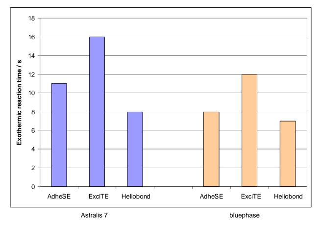
Fig. 21: Exothermic reaction times for AdheSE, ExciTE and Heliobond during light curing with Astralis 7 and bluephase (Low Power mode) (R&D, Schaan, 2007)
