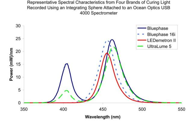
Fig. 5: Wavelength range and light output of bluephase compared to three other LED lights measured with an integrating sphere (Price, Halifax, 2007)
