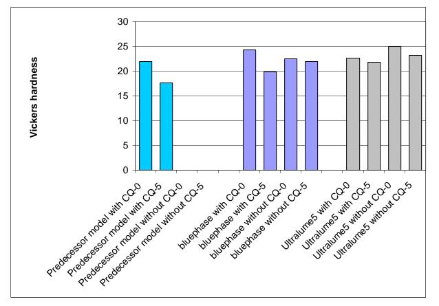
Fig. 19: Curing of the ExciTE adhesive with and without camphor quinone after a curing time of 10 seconds using the Low Power mode with a distance of the light guide of 0 and 5 mm. Measurement of the Vickers hardness. (Ilie, Munich, 2007)
