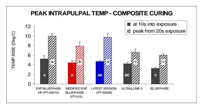
bluephase 20i has been tested using the same test conditions.
