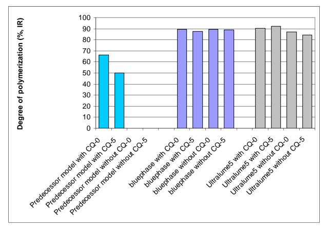
Fig. 18: Curing of the ExciTE adhesive with and without camphor quinone after a curing time of 10 seconds using the Low Power mode with a distance of the light guide of 0 and 5 mm. Measurement of the double-bond conversion using ATR-IR (Ilie, Munich, 2007)
