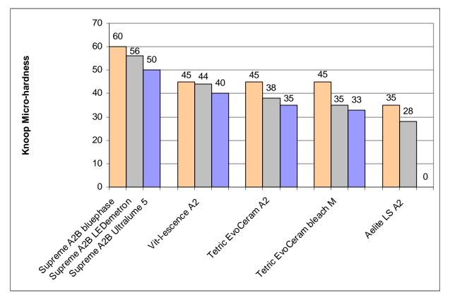
Fig. 12: Micro-hardness on the bottom surface of five different composites after having been exposed to the light of bluephase (orange), LEDemetron II (grey) and Ultralume 5 (blue) for 10 seconds at a distance of 4 mm from the light guide (Price, Halifax, 2007)
