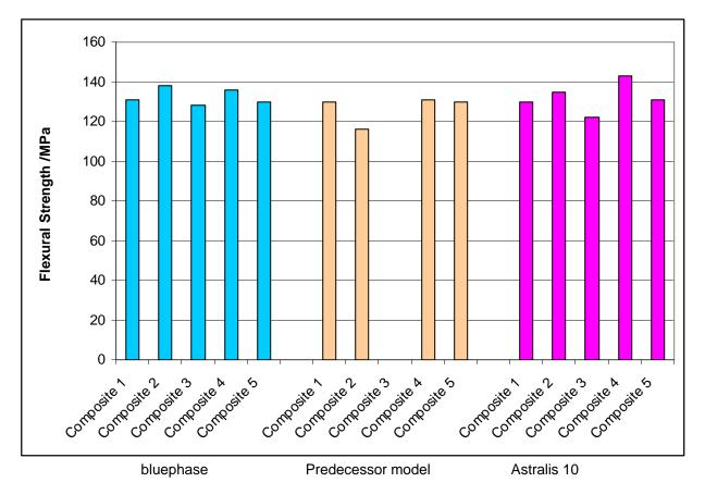
Fig. 17: Flexural strength of different experimental composite formulations with different initiator contents (see Table 2) after having been exposed to the light of the predecessor model, bluephase and Astralis 10 for 20 s using the High Power mode. (R&D, Schaan, 2007)
