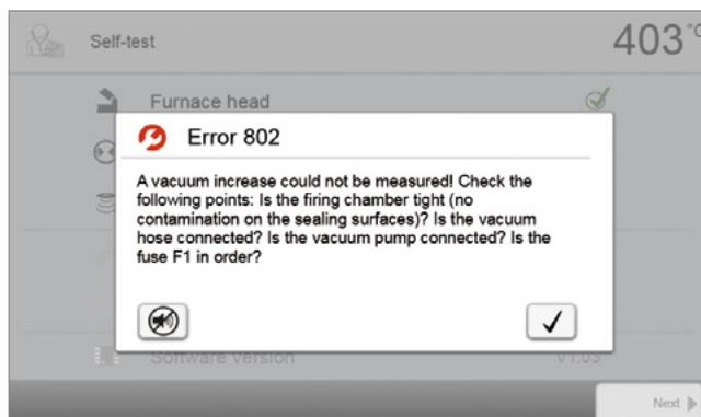
The acoustic signal and the error message can be acknowledged with the corresponding buttons.
