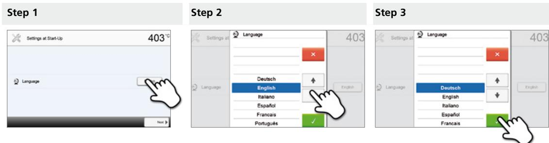
Select the desired language using the **[arrow up/down]** buttons. Confirm the entry with the green button. By pressing the **[Continue]** button, you will reach the next entry screen.
