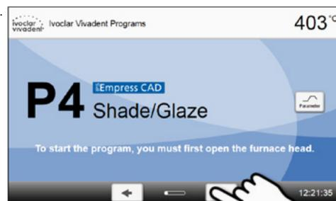
The **[Parameters]** button is used to switch to the program parameter screen. Firing programs can be edited in this screen
