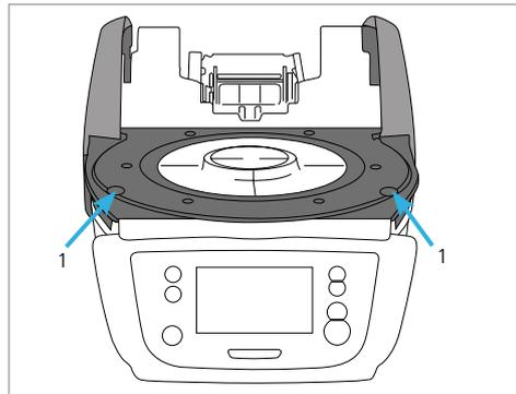
Place the cooling tray (2) on the frame plate (24). Make sure that the cooling tray is correctly positioned on the frame plate.
