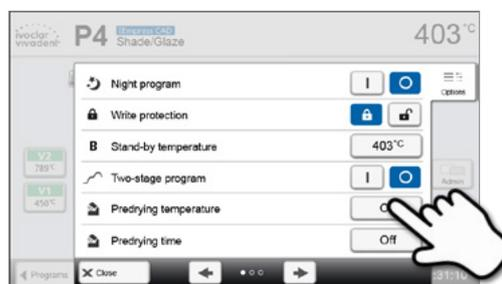
3. Enter the desired predrying temperature and confirm with the green button.
