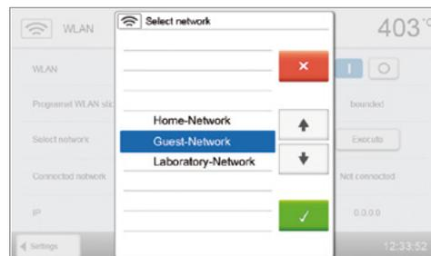
**4. Enter the WLAN password and confirm with the green button or abort the entry with the red button.**
