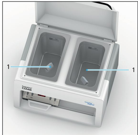
3. Keep the lid open and fill both cleaning containers with cleaning fluid up to at least the lower fill level mark and at the most to the upper fill level mark (2) (min. / max. fill level).
