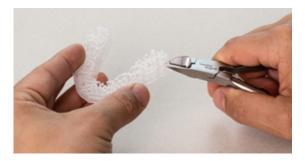
Manually breaking off the support structures is not recommended as this may cause tears on the objects!
